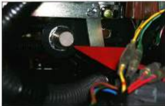
• Proximity sensor For prevention from drop of the mower (plot plan drawing 1)
